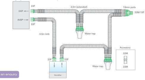
CodeDescriptionBox Qty.215500022mm Compact, extendable breathing system with two re-sealable water traps and 1.5m limb, 3.0m12
