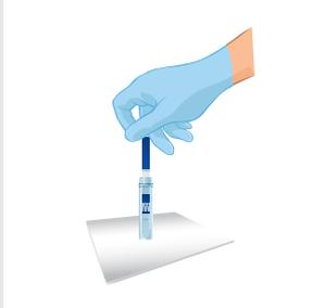
3. Test strip is inserted into vial and removed when two lines are visible, or at 10 minutes
