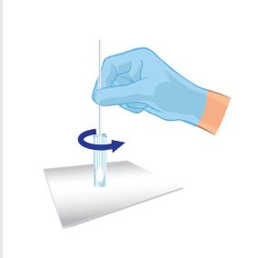
2. Swab is rinsed in vial with solvent and then disposed of
