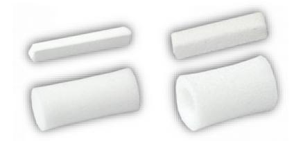
In the picture above: delivery condition (dry) In the picture below: expanded state (wet)
