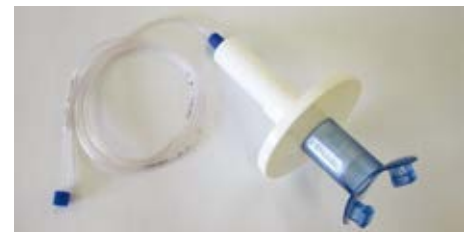
MIP/MEP Pressure Transducer with antibacterial filter and rubber mouthpiece
