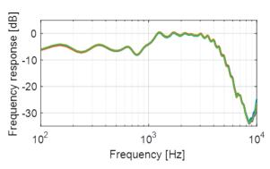
Frequency response measured of an IP30 in a 711 coupler using the Sanibel  $^{\rm TM}$  insert foam tip
